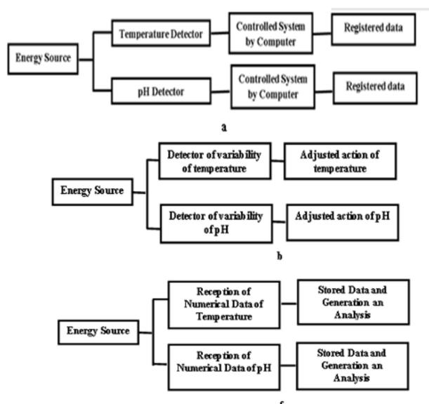
**Fig-4:**Automatization system to control physicochemical factors constituted by (a) Principal system, (b) Adjusted System and (c) Registration data values
